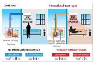
\* Defrost operation time and how low room temperature falls differ depending on the environment in which the unit is being used (how insulated and airtight and room is), operation conditions, and temperature conditions.
